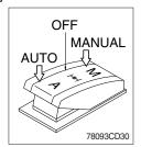
(1) This switch is used to apply differential lock. The differential lock gives equal power to both rear wheels and is used in conditions when traction is poor.
