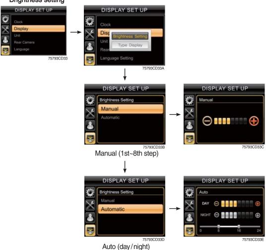
If "Automatic" is chosen, brightness for day and night can be differently set up. Also by using the bar in lower side, users can define which time interval belongs to day and night. (in bar figure, gray area represents night time while white shows day time)
