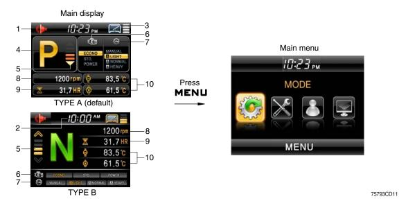
1 Buzzer 5 Select gear 9 Hour meter, odometer
